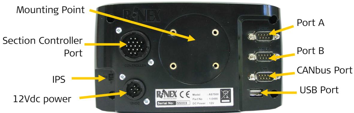
**Figure 3-4 AS7500 controller rear panel and connectors**
