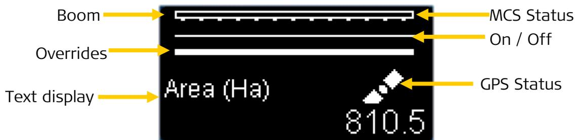
**Figure 3-6 AS7500 display panel in Operational Mode**
