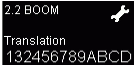
As an example if a five section boom had two additional switches placed for further control of the two outer most sections as shown in Figure 3-9 then it would be necessary to translate which sections would be activated by the AS7500. In this example it would be necessary to have the translation as shown in the sequence beneath the boom in Figure 3-9.
