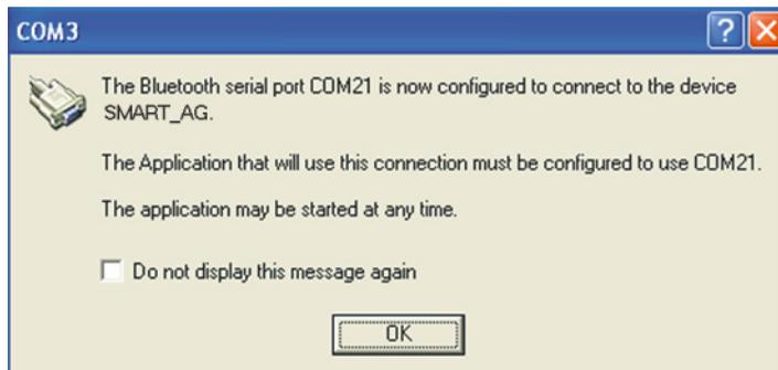
**Figure 25: Computer Bluetooth Port Assignment**
